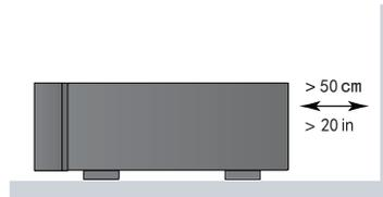
**WARNING:** The rear panel power cord connector is the mains power disconnect device. The device must be located in an open area that allows access to the cord connector.
