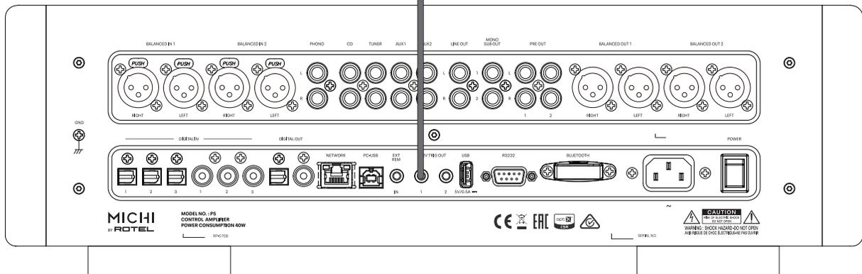
Figure 5-2 : 12V Trigger Connections
