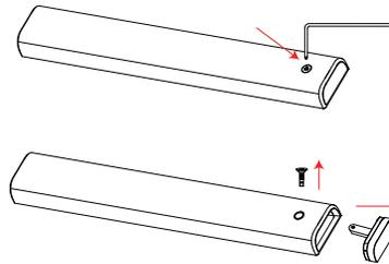
3. Install the batteries as shown in the illustration in the battery well (Figure 2). Please note there are negative and positive marks shown on the battery cover (Figure 1). Reassemble the battery cover and tighten the screw then test the control for proper operation.
