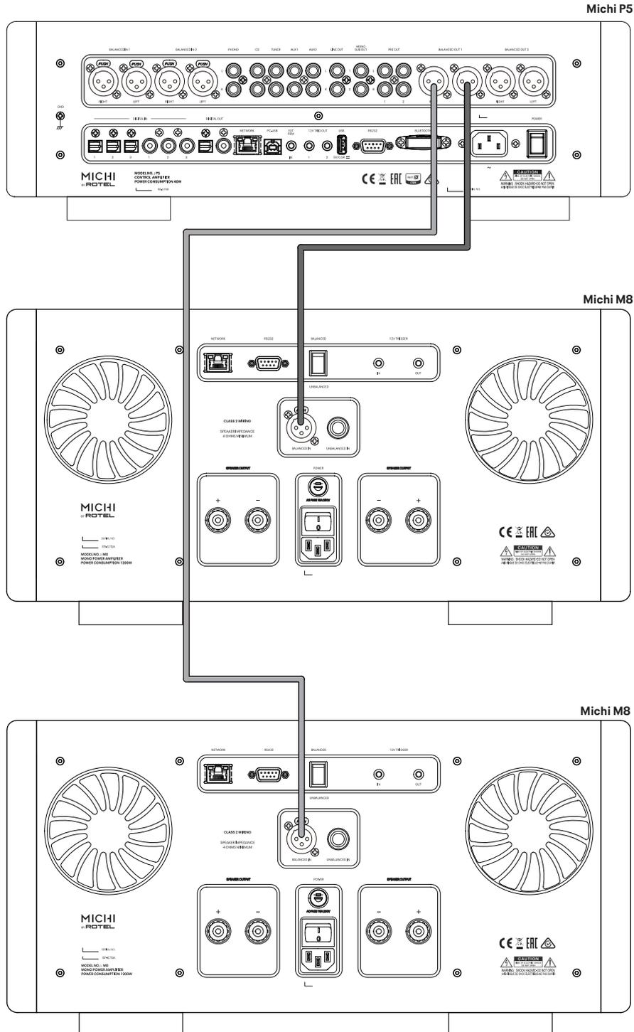
**Figure 5-1 : 12V Trigger Connections**
