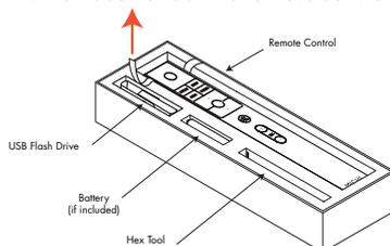
2. Remove the screw on the back of the remote using the hex tool provided with the remote. Use only the hex tool supplied to avoid damaging the attaching screw.
