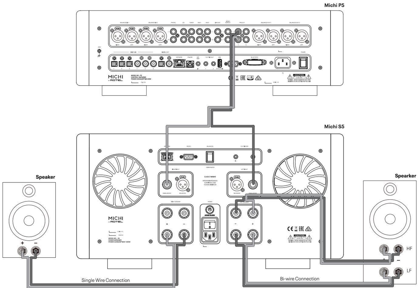
Figure 3-2: Analog Input and Speaker Output Connections
