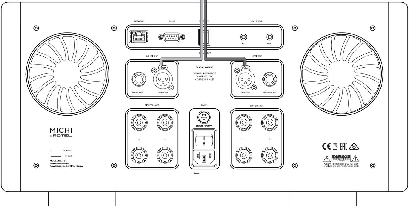
**Figure 4-2: Balanced (XLR) Inputs Connection**
