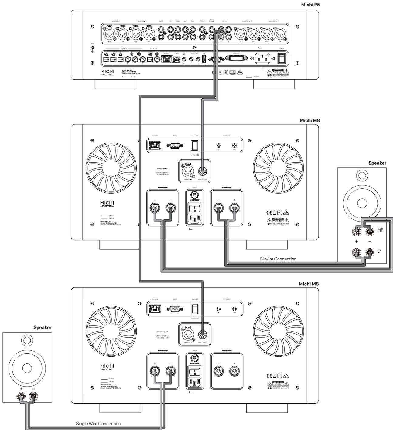
**Figure 4-1 : Balanced (XLR) Inputs Connection**
