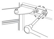
2 Rotate the hinge out of the way so that the door can be lifted off.
