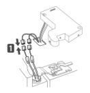
4 Make sure that the door-switch located inside the cover is tightly connected. Position the cover in its place. Insert and tighten the cover screw 2.
