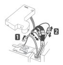
4 Rotate the hinge lever counterclockwise 1. Lift the top hinge 2 free of the hinge lever latch.
