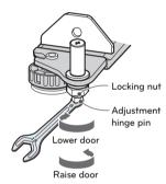
(3) After the door heights are adjusted, completely tighten the locking nut by turning it ( ✓ ≯) counterclockwise.
