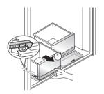
3 Support underneath the glass cover with one hand while lifting the front of the cover with the other hand. Push up from underneath to release the cover from the guides, then tilt the cover 45 degrees, and pull it forward to remove it.
