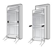
2 Lift the front of one drawer to remove it from its guides and pull straight out. Repeat to remove the second drawer.
