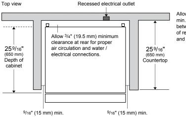
Allow 2" (50 mm) min. clearance between the top of refrigerator and alcove.
