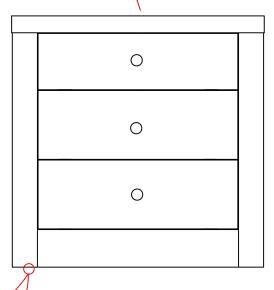
Adjust leveler if needed to level nightstand on uneven floor.
