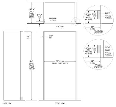
NOTE: 31/2\* (89) finished returns and shaded areas will be visible and should be finished to match cabinetry. Shaded line represents profile of unit with 3/4" (19) panel.
