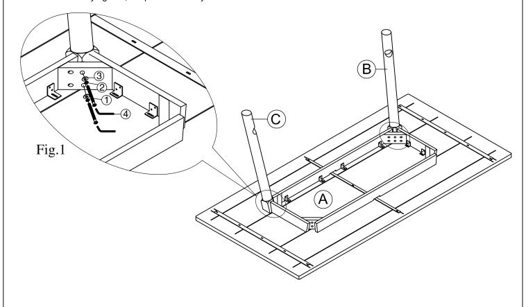
STEP 2: Attach iron frame (D) to table leg (B) and table leg (C)
