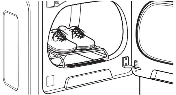
3. Place wet items on top of the drying rack. Allow space around items for air to circulate. The drying rack does not move, but the drum will rotate; be sure to leave adequate clearance between items and the inside of the dryer drum. Make sure items do not hang over the edges or between drying rack grille.
