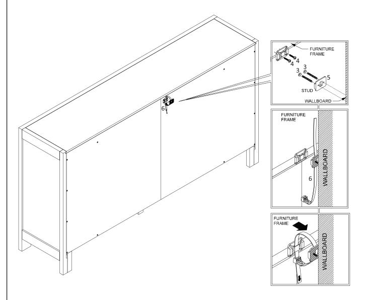
**STEP (A)** Locate a wall stud behind your furniture. Position a bracket on the stud approximately 1'' below the top of the furniture. Mark & drill pilot hole into the center of the stud with a 3/32" drill bit. Attach the bracket to the stud with the screws provided (3).
