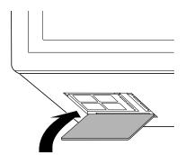
**4** To reinstall the grease filter, insert the back of the filter, push the filter toward the back, and lift the filter up into place.
