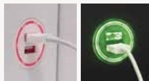
Dual USB Charging Ports (red = charging, green = fully charged)
