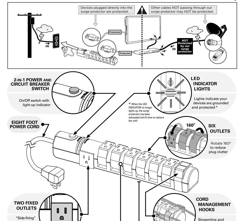
**COMPONENTS:** • 2160J Surge Protection w/ Max Spike current 144,000A or 6KV • Clamping Voltage: L-N 330V, L-G 400V, N-G 400V (3 lines of voltage protection)
