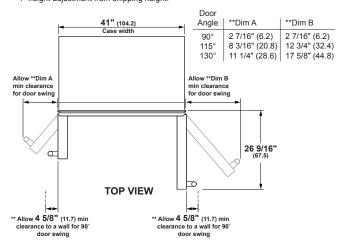
\*\* These refrigerators are equipped with a 3-position door stop. The factory-set 115° door swing can be adjusted to 90° if clearances to adjacent cabinets or walls is restricted. Allow full 130° door swings for pan removal. If the 90° door stop position is used, pan access is maintained, but pan removal is restricted.
