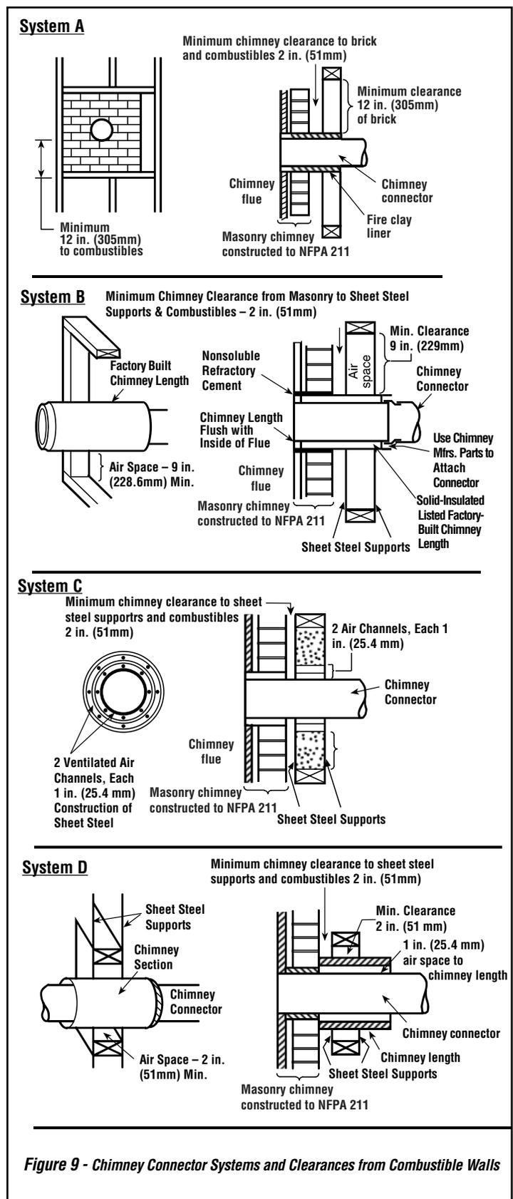
**Figure 9 - Chimney Connector Systems and Clearances from Combustible Walls**
