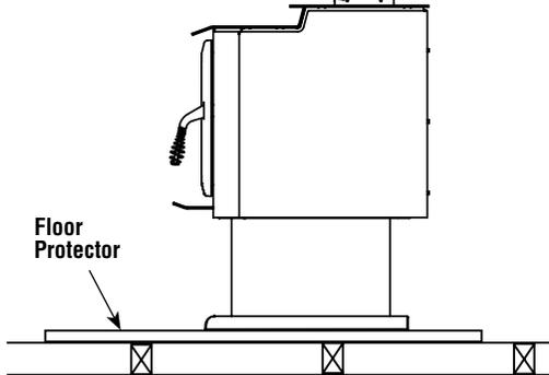
**Figure 6 - Typical Installation**
