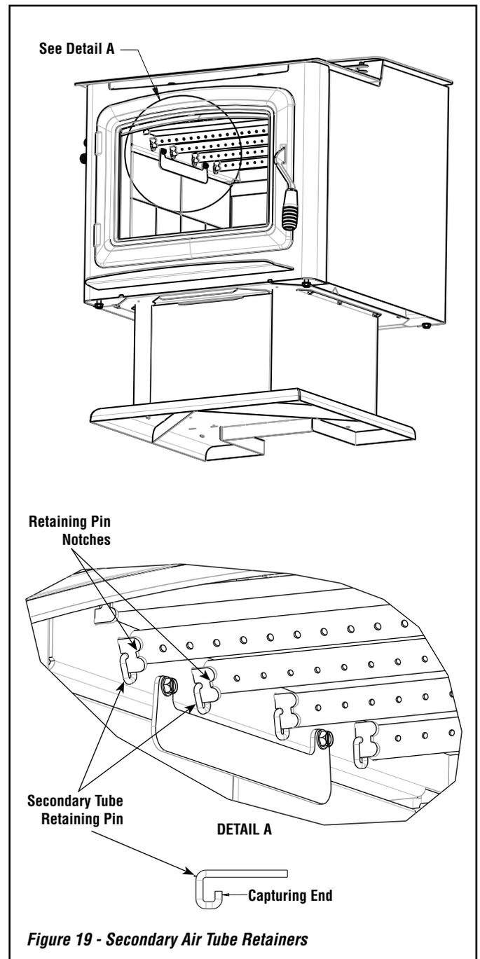
Figure 19 - Secondary Air Tube Retainers
