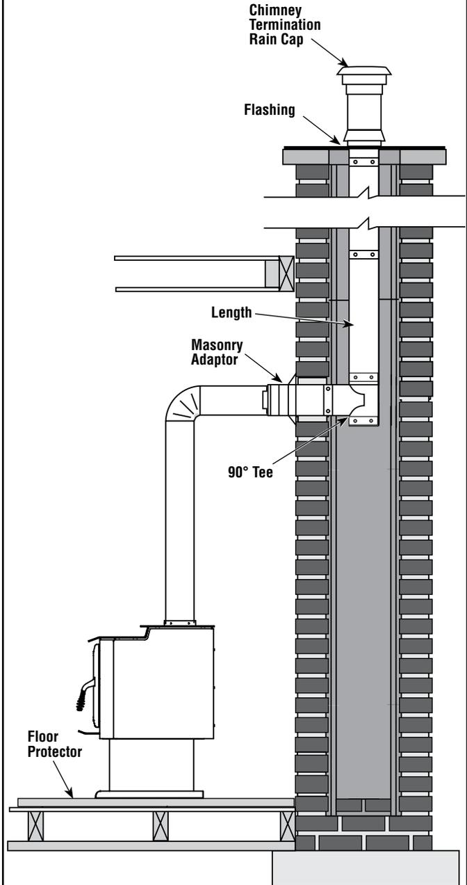
**Figure 7 - Connected to a Masonry Chimney**
