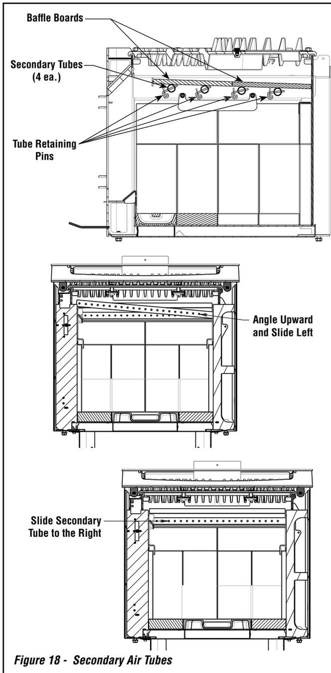
Figure 18 - Secondary Air Tubes
