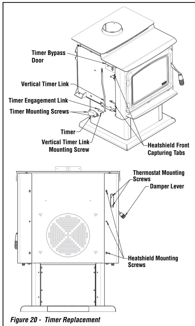
**Figure 20 - Timer Replacement****POST INSTALLATION CHECKS**
