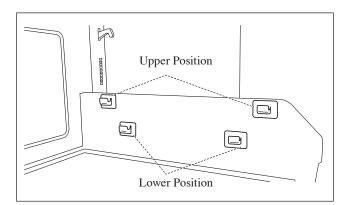
Use the correct accessories provided for each cooking mode. Place accessories in the correct installation position and direction.
