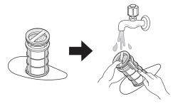
To replace the assembled filters, position the spray arm so the wider vee is toward the front. Fit the filters back into the filter holder
