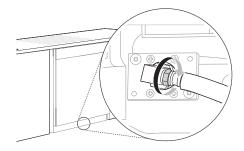
Slide the water supply line back through the channel, pulling gently from inside the cabinet to make sure the line is not kinked, pinched, stressed or crushed.
