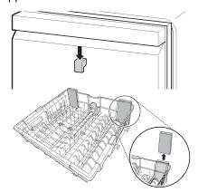
Press the tab to remove the cable tie by hand.
