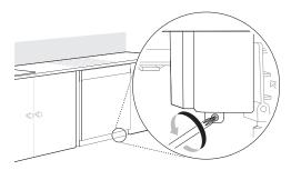
Use a Phillips screwdriver to remove 2 screws0.
