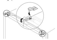
Bend the tabs on the brackets to secure them to the frame using a pair of needle nose pliers.
