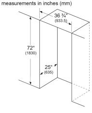
Leave 2" (50.8) gap at the top and 1 3/8" (34.9) behind the refrigerator for proper ventilation.
