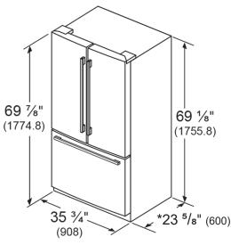
\* Add 1 3/8" (35) in the back measurements for proper ventilation
