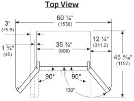
Drawers can be pulled out with door open to 90°. Drawers can be taken out with door completely opened.
