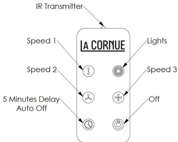
The diagram to the left shows all functions of the remote. Push the speed or light buttons once to turn on; push the same button a second time to turn off. You can use the "off" button to power off the lights and blower simultaneously.
