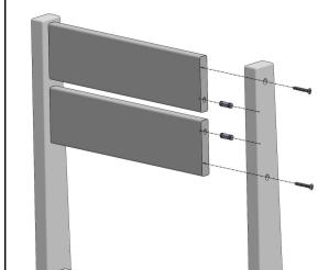
Tap 5/16" dowels into large holes in back slats. Align with large holes in rear legs. Secure with 1-3/4" Phillips head screws through 3/8" counter-bore in rear legs into pilot holes in back slats.
