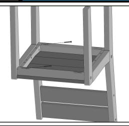
At this time make sure lags from step 2 are tight. Rotate rear apron to align with angle on seat support, and make sure front apron is parallel with front leg. Secure aprons with 1-3/4" Philips head screws through the pockets on underside of aprons into legs.
