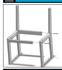
Attach front and rear aprons to Side assemblies as shown, with the pockets of the aprons facing down using (4) 80mm Hex Lags.
