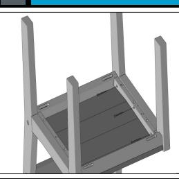
Align seat assembly with frame. Secure using 1-3/4" Philips head screws through countersink holes on inside of seat assembly into pilot holes in side assemblies.
