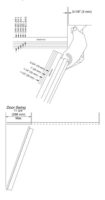
**NOTE**: Additional space needed depending on the thickness of front panels and handle used.
