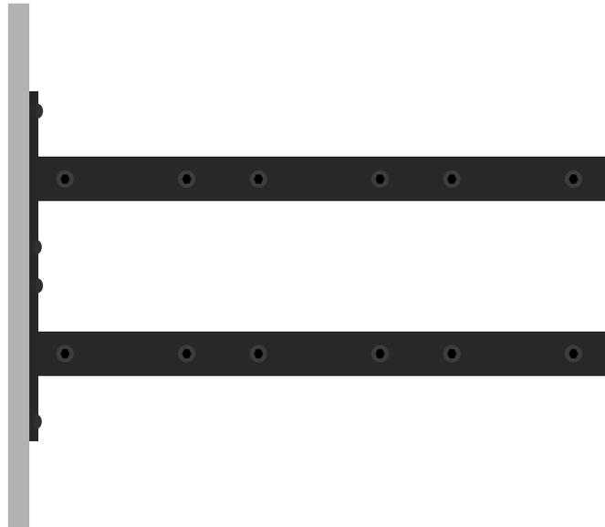
Multi-rack installation: Leave a minimum 3in (8cm) gap between the rack brackets to ensure there is enough room for bottles. You can also put the rack brackets closer together, but it will be hard to pull out the bottles from back row if you do so.
