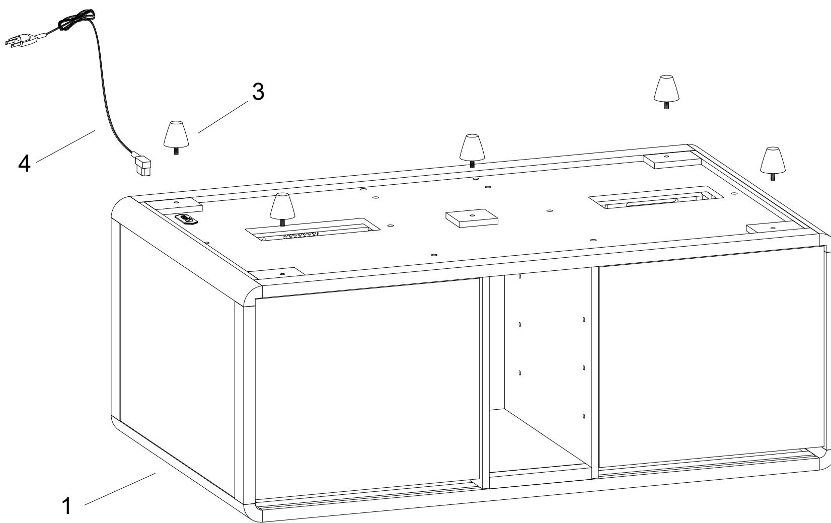
**Step 2: Return TOP BOX(1) to the floor, and Insert PANEL(2) into the TOP BOX(1) as shown.**
