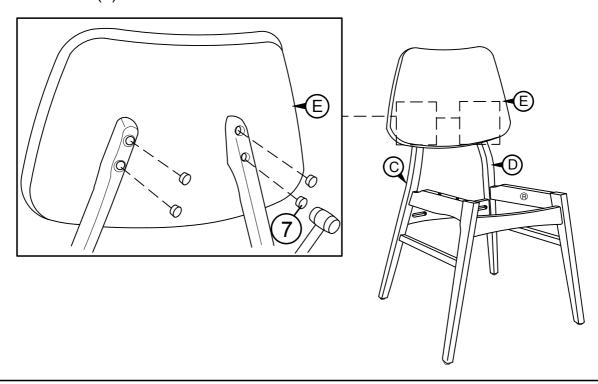
STEP 5: To level the chair, place the chair on a flat surface and tighten all the bolts using Allen Key (3).
