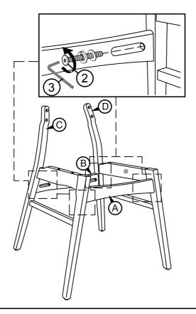
STEP 3: Assemble the Chair back (E) to the top of the assembled chair frame by using the Allen Key (3) with the hardware 1.
