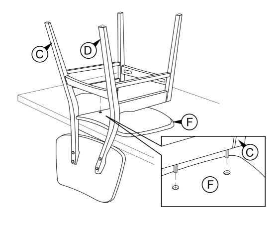
STEP 8 : Assemble the seat frame (C&D) to the Cushion Seat (F) by using a screwdriver with hardware 4 and 5.
