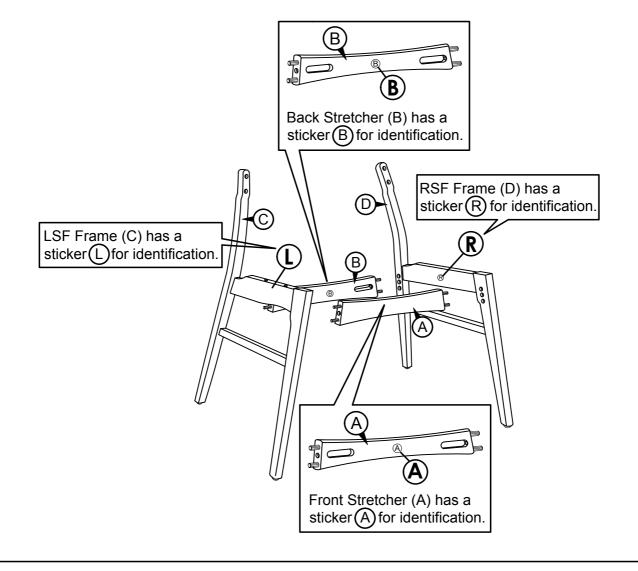
STEP 2: Assemble the front stretcher (A) and the back stretcher (B) to the LSF Frame (C) and RSF Frame (D) by using the Allen key (3) with the hardware 2.
