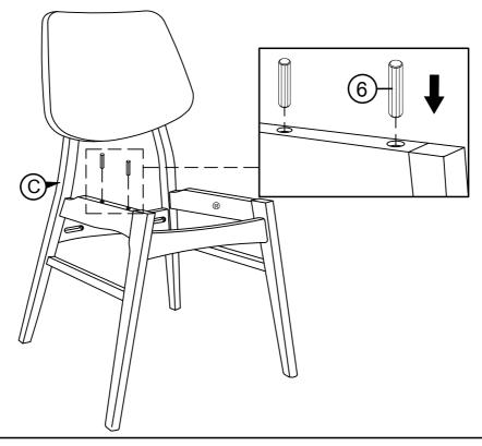
STEP 7: Place the Cushion Seat (F) bottom-side up on a elevated surface (e.g. table top). Then place the chair frame upside down so the wood dowels on the LSF frame (C) are positioned into the Cushion Seat (F).
