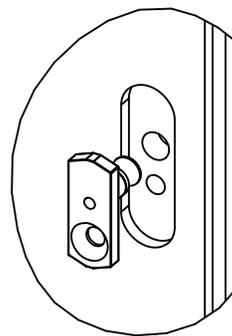
Tighten the set screw in the handle cap after tightening screw D
