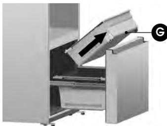
4. Remove the lower freezer drawer (C) by lifting it up.
