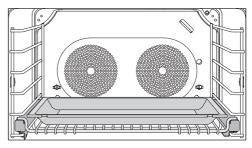
You can also place the universal tray directly on the FlexiClips with wire rack.
