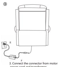
3. Connect the connector from motor to the power cord and transformer
