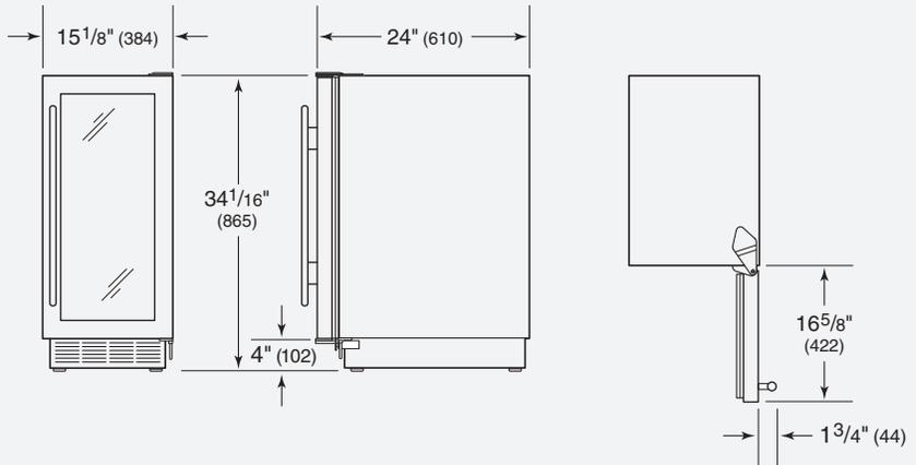
Overall dimensions are based on stainless steel panels and handles.
