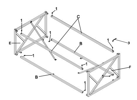
STEP 2: 1.Attach Top/Bottom Rail (B,C) to Left/Right Side Frame (E,F) using Bolt (1) and tighten bolts with Allen Key (3).
