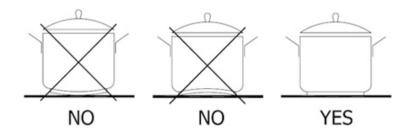
Each cooking zone is equipped with a "pan present" device, which ensures that cooking cannot start unless a suitable pan is placed on the cooking zone and properly positioned.
