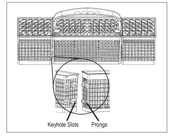
The three separated modules of the silverware basket can be used in both Upper and Lower Racks.
