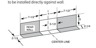
electrical outlet box. Recommended outlet locations allow range
