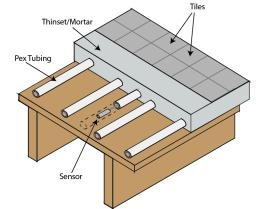
The SLAB sensor is embedded into the bed of mortar or concrete and centered between two rows of pex tubing. It is recommended that the sensor be installed into a length of pex tubing or metal conduit to protect it during installation and if the sensor ever needs to be replaced, it can be removed and installed easily. The above illustration is just one method used to install the slab sensor. Depending on the type of floor and system being used, installation procedures can vary
