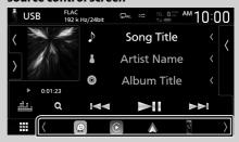
Display source selection buttons by touching / Dor flicking left or right on the source control screen, then select a playback source.
