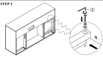
\*Note: Slightly move the speaker forward and install the wood stretcher on the back side of the case (top and bottom).
