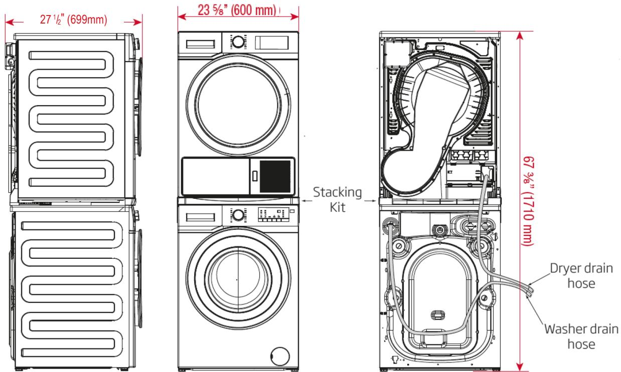
**Stacked installation minimum air gap clearances:**
