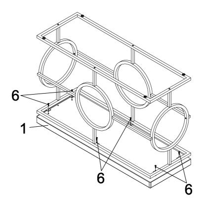
Step 5: Attach the assemble in Step 4 to Mirror Box (1) using Short Bolt (6) as shown.
