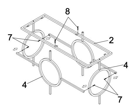
Step 2: Attach Large Frame (4) to the assemble in Step 1 using Medium Bolt (7) and Long Bolt (8) as shown.
