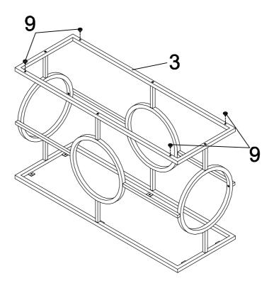
Step 4: Insert Leveler (9) onto Bottom Frame (3) as shown.
