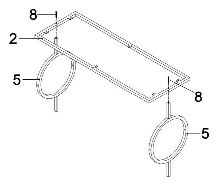
Step 1: Attach Small Frame (5) to Top Frame (2) using Long Bolt (8) as shown.
