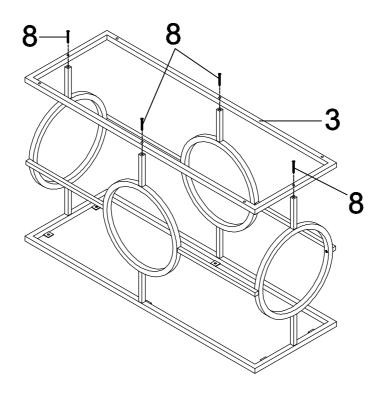
Step 3: Attach Bottom Frame (3) to the assemble in Step 2 using Long Bolt (8) as shown.
