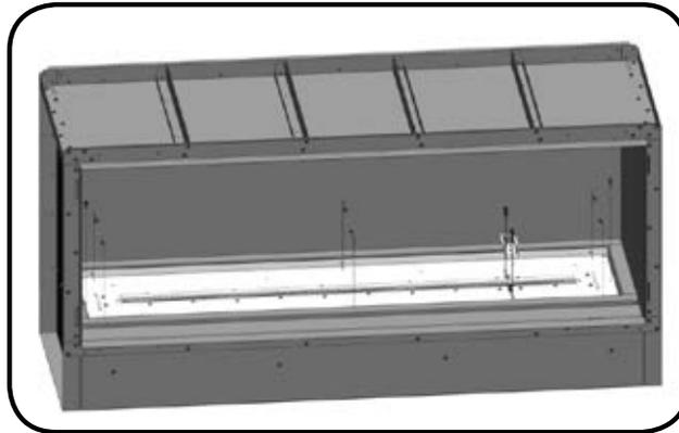
Lift the glass tray from the fireplace, pushing from the top, disengage the thermocouple and igniter from the glass tray.
