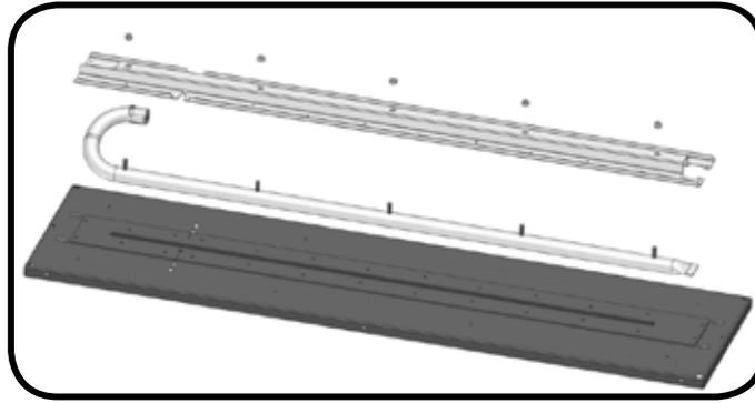
**Reinstallation:** Reverse the procedure to reinstall the burner ensuring that the holes on the gasket between the burner bracket and glass tray are lined up during re-assembly. Check that the orifice enters the burner when installing. Replace the glass embers and the front glass shield. When the appliance is put back in service, check the burner flame pattern with the image below.
