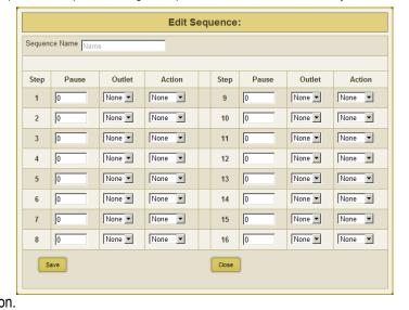
\*Time delay is specified from the previous sequence item, not from the initial starting point. For example, creating a sequence with "Step 1, 1 second, Outlet 1, On" and "Step 2, 1 second, Outlet
