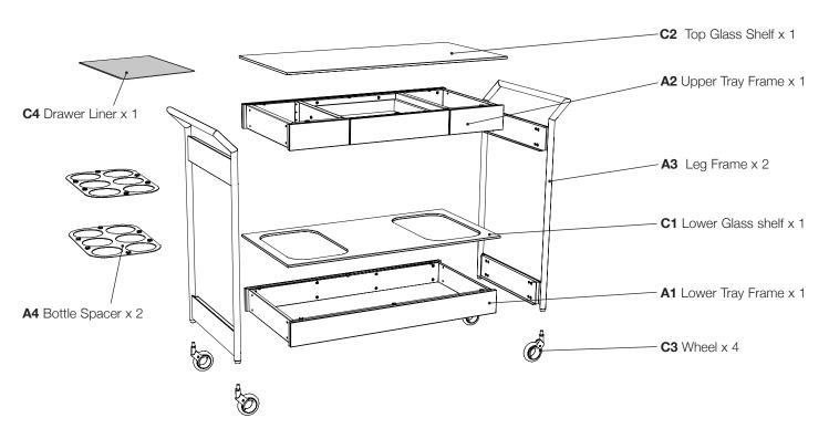
Insert 6 rubber stem bumpers H2 into the holes along the top edges of the upper tray frame A2.
