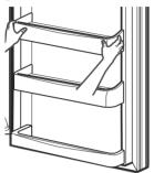
**2** To assemble the bin, slide it in above the desired support and push down until it snaps into place.
