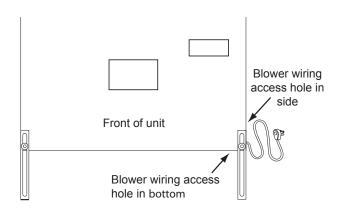
WIRING/CONDUIT CONNECTIONS FOR REMOTE/IN-LINE BLOWER
