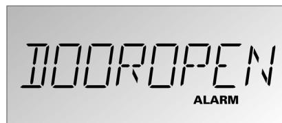
Close the door to switch off the warning signal.
