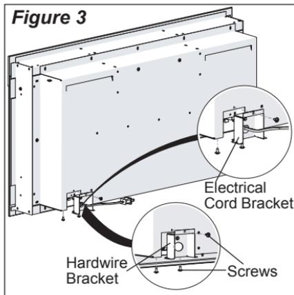
cord bracket from the back of the fireplace by removing the three retaining screws. (Figure 3)
