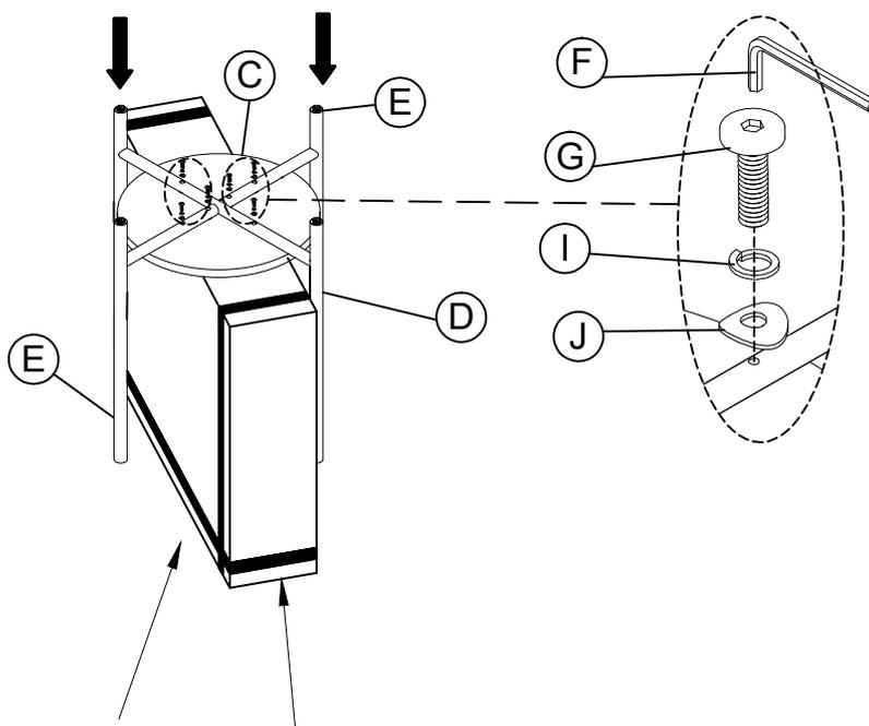
**Attention:** When attaching all legs to the shelf, use the carton from the packaging or a work surface to create a gap between the floor and the legs. This will allow the legs to easily be assembled and properly tightened.
