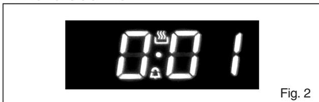
As this minute counter does not control the oven, when it finishes counting the oven will continue to work.
