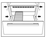
Install the combination appliance in accordance with its own specific operating and installation instructions. The front panel must be at least  ${}^{3}/{}_{4}{}^{"}$  (19 mm) thick and be temperatureresistant up to 140°F (60°C). The decorative front, including the handle, may not exceed a weight of 11 lbs. (5 kg).
