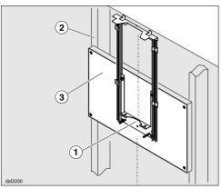
■ Determine and mark the location of the retaining plate ① for the canopy as outlined on the "Installation diagram".
