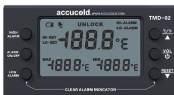
Your appliance is equipped with a NIST calibrated temperature monitoring device (TMD) also referred to Thermometer/Alarm that simultaneously displays minimum, maximum, and current interior temperatures and provides a visual and audible signal when the temperature inside the unit falls outside the set temperature range.
