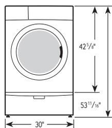
Required Dimensions for Installation with Stacking Kit
