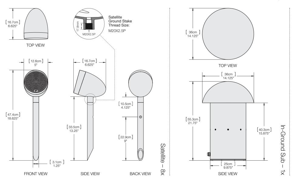
OVERALL SATELLITE DIMENSIONS: (H) 18.625" [47.4cm] x (W) 5" [12.6cm] x (D) 6.625" [16.7cm] OVERALL IN-GROUND SUB DIMENSIONS: (H) 21.75" [55.3cm] x (W) 14.125" [36cm] x (D) 14.125" [36cm] SATELLITE WEIGHT: 3lbs (1.4kg) each IN-GROUND SUB WEIGHT: 17.7lbs (8kg) each
